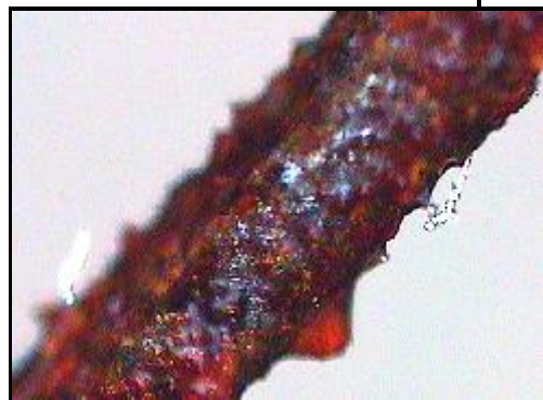
Breather Filter Media Support Aluminium Mesh @ 100X/200X
