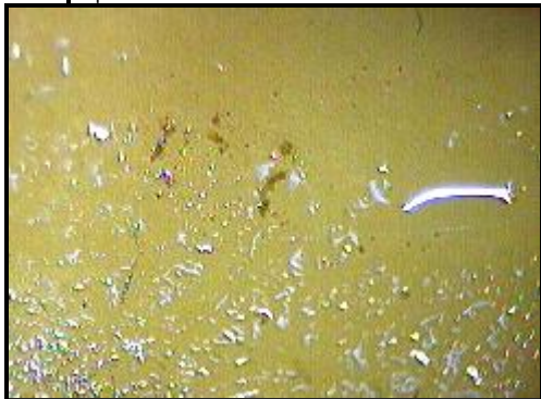
3µm Membrane Filter Breather Filter Media
