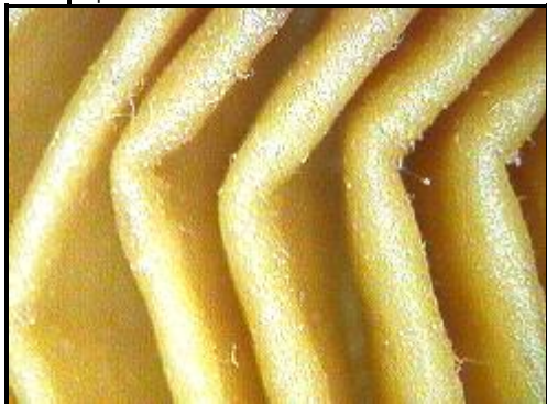
3µm Membrane Filter Breather Filter Media
