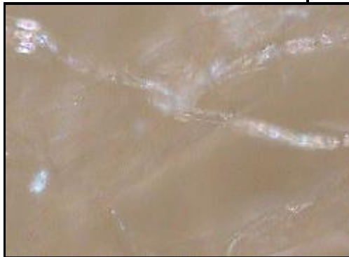
Breather Filter 3 µm Inner Media Close Up @ 100X/200X
