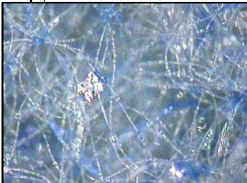
3µm Membrane Filter Breather Filter Media
