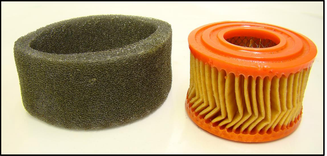
The Outer Foam Pre Filter and the pleated particulate filter were both heavily saturated with lubricant
